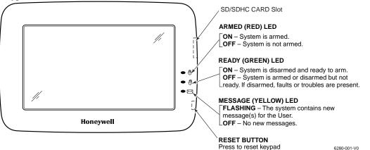
**NOTE:** If the Screen Blackout (\*EN50131 Display) feature is enabled (see below) the keypad returns to the "Home" screen and the "Armed" and "Ready" status LEDs turn OFF after 30 seconds. The keypad will remain in this state until a valid user code is entered.
